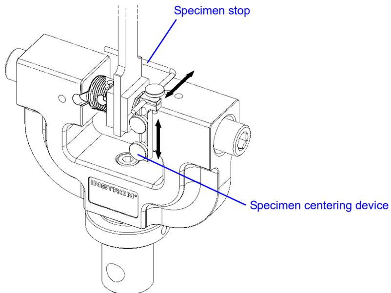
*Figure 4-2. Using the Specimen Centering Device*
