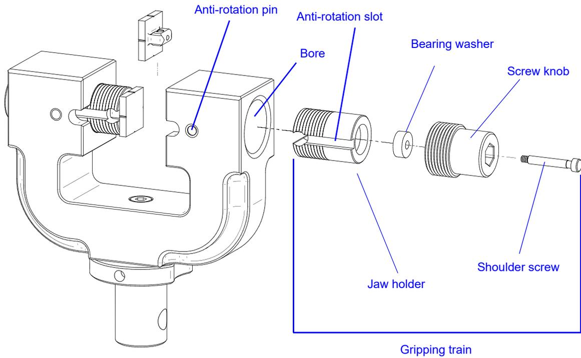
*Figure 5-1. Lubricating the Screw Knobs and Replacing the Bearing Washers*
