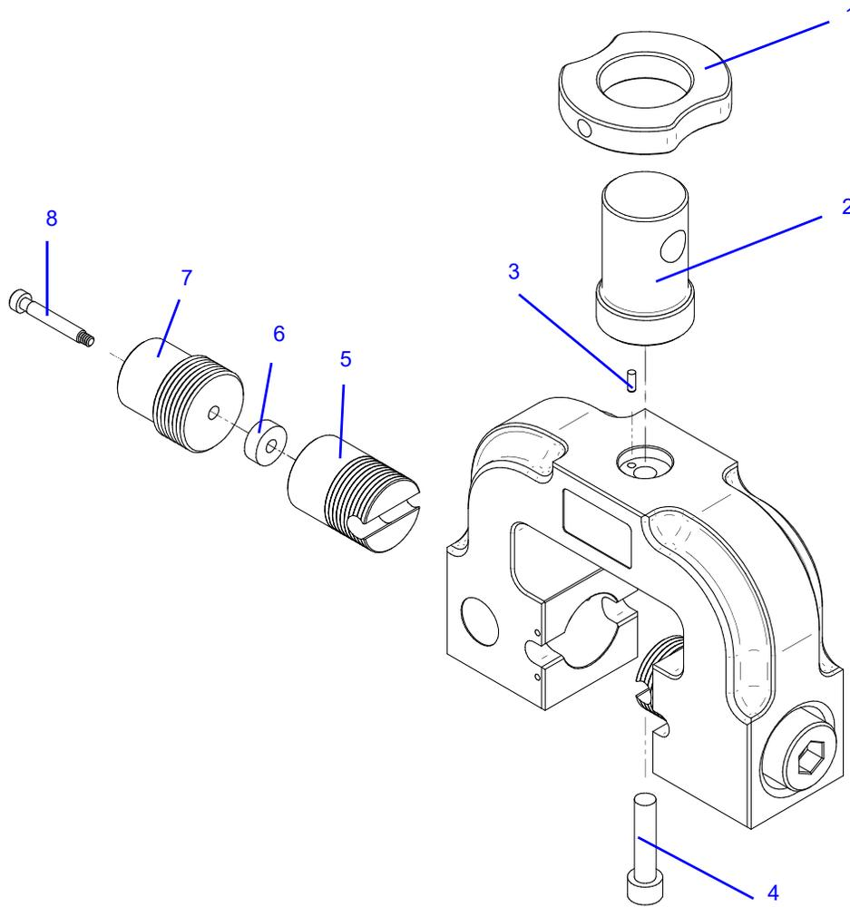
Figure 6-1. Exploded View of 2710-115 (5kN) Screw Action Grip
